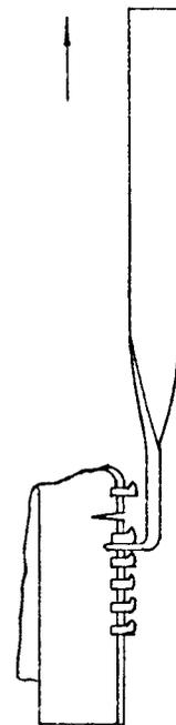
FIG. 2 Fixture for Element Slippage Test
