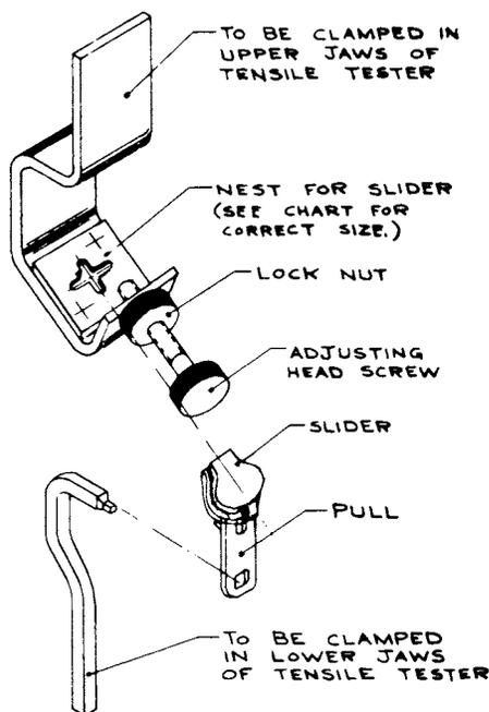
FIG. 20 Fixture for Angular Pull, Pull-Off Test
