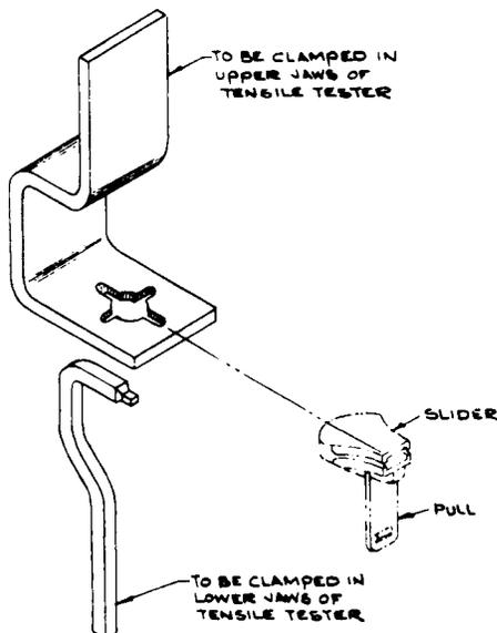
FIG. 19 Fixture for Slider Pull, Pull-Off Test
