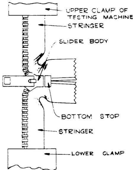
FIG. 7 Bottom Stop Holding, Stringer Separation Test
