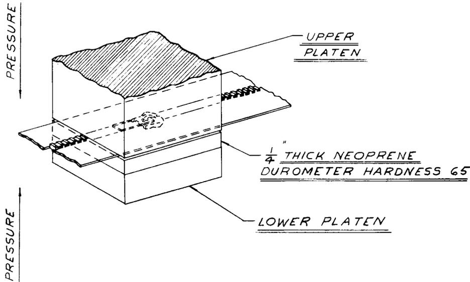
FIG. 13 Test for Slider Resistance to Cushioned Compression
