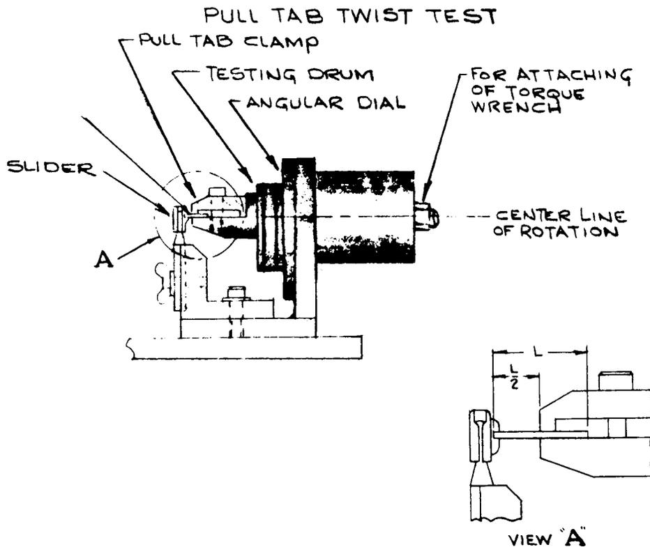
**FIG. 18 Apparatus for Twist for Slider Pull Tab**
