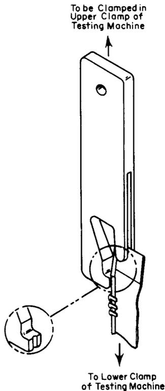
**FIG. 9 Fixture for Separable Pin Pull-Off Test**
