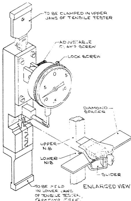
**FIG. 14 Fixture for Slider Deflections Test (Mouth)**
