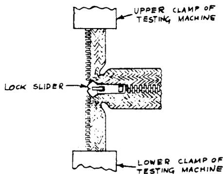
**FIG. 21 Slider Lock Holding, Stringer Separation Test**
